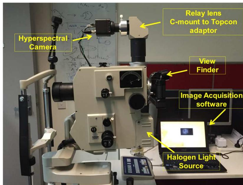
Figure 1: Hyperspectral fundus imager (Camera Setup)
